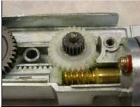
8. Re-install the 2nd drive gear as shown.
