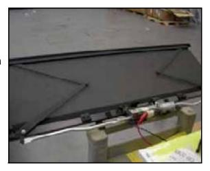
3. Begin disassembly of the motor gear box by using a heat gun to soften the thread locker used to retain the (2) screws. Heat should be applied to the (2) screws and the immediate surrounding area at least for 40 seconds to ensure the screws are free from thread locker material.
