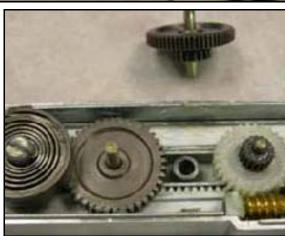
6. Remove the old plastic gear by pulling it straight up and out.
